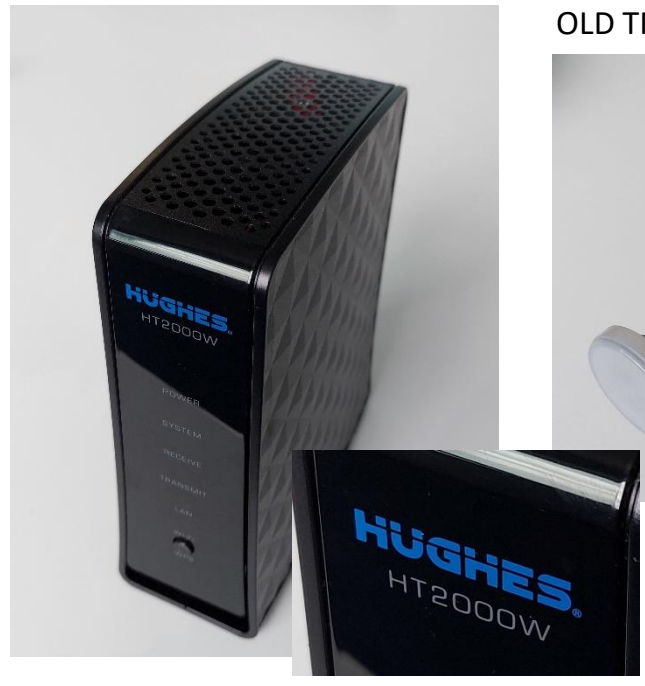
MODEM INSIDE TERMINAL
