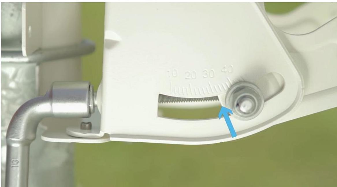
Once the elevation is set, proceed with moving the dish in the direction towards the azimuth results until you notice the 'beeps' become faster and higher pitched, keep moving in this direction until you reach a solid tone, this will indicate that you have locked on to the satellite.
